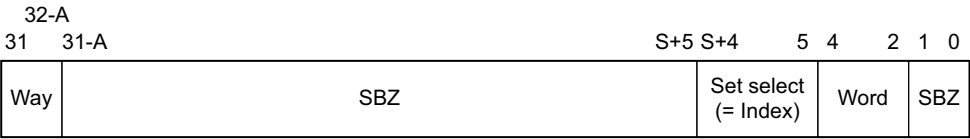
Figure 4-3 ARM926EJ-S cache Set/Way/Word format
